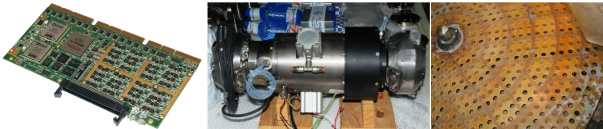
Figure 8 – Main components: Adopt 16ch DSP control board (Microgate), hexapod leg (ADS), reference body (SESO)
